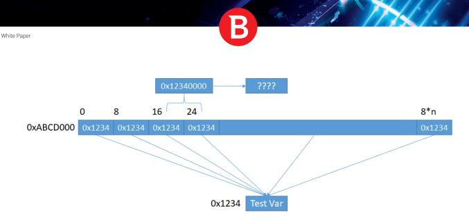
Figure 2. A misaligned load would access other locations, instead of the test variable
